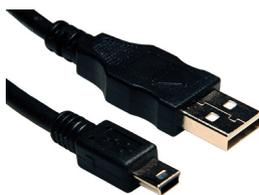
Shielded Universal Serial Bus (USB) cord compatible with USB 2.0. Fitted with USB-A plug to Mini USB-B plug. Two x 28AWG (signal) and 2 x 24AWG (power) conductors.
