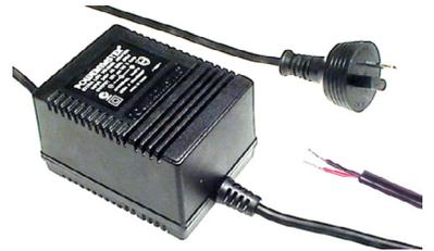
In-line AC adaptor has 24 Watt maximum capacity with output voltages from 3V to 30V with 500mA to 5 Amp current range. The AC input cord fitted with mains plug has insulated pins compliant with AS/NZS3112. Dimensions 67(L) x 59(W) x 88(H)mm. Electrical Safety Authority Approved.
