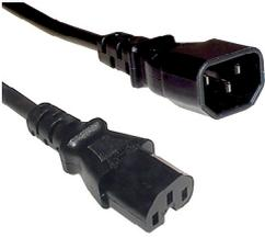
A 10 Amp AC power cord used mainly to power computer servers from a UPS IEC outlet. Fitted with male IEC-C14 and female high temperature IEC-C15 connectors. High temperature RR flex as required for compliance when molded to the IEC-C15 connector.
