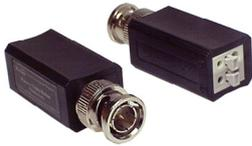
Used to carry CCTV video signal over Cat5e or Cat6 cable. Passive design transmits colour video up to 400 metres. Male BNC for video connections and either push-pin or screw connection to the Cat5e or Cat6 cable. Blister pack set of two.
