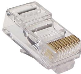
Generally used on cellular mobile transceivers and small multi-line telephone systems. Plugs with 50µ" or 30µ" gold plated contacts are available. Packed in bags of 20, 50, 100 or 1000. Plugs for stranded or solid conductors are available.
