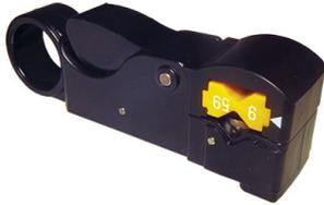
For stripping RG6/U and RG59/U coaxial cables. 3 blades ensure accurate stripping length of each cable section. Built-in hex screws for accurate depth-of-cut adjustment for each blade. Preset stripping length of 12mm (8mm + 4mm). Blades may be repositioned to give a 10mm (6mm + 4mm) stripped length. Reversible cutting block for quick change when stripping between RG6/U and RG59/U coaxial cables.
