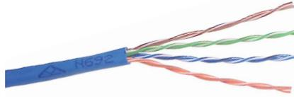
Now available in Reel In Box, quality Cat5e Solid conductor cable using 100% bare copper. 4 twisted pairs 24AWG with 7/0.02mm<sup>2</sup> solid copper conductors. Capable of supporting up to 100Mbps @ 100MHz and reduces the amount of crosstalk, resulting in a greater overall transmission speed. Available in 10 colours, with count down metre marking. Custom branding and colour also available.
