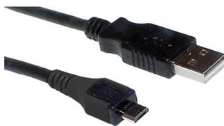
Shielded Universal Serial Bus (USB) cord compatible with USB 2.0. Fitted with USB-A plug to Micro USB-B plug. Two x 28AWG (signal) and 2 x 24AWG (power) conductors. Commonly used on recently released mobile phones, PDAs and other handheld devices for data connection to a PC and/or battery charging.
