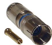
Datamaster's high performance female PAL compression connector for trouble free professional water-proof coaxial connections. Blue colour coded band indicates compatibility with RG6/U quad-shield coaxial cable. Attach using our coaxial cable stripper and professional ratchet compression connector crimp tool T0040.
