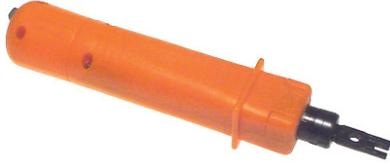
Quality impact tool for 110 type IDC terminations. Adjustable tension for impact mechanism. Reversible blade allows terminate only or terminate/cut operations. On-board storage of spare blades. Replacement/spare blades are also available. Not suitable for Krone type IDC terminals.
