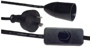
Light duty 10 Amp 2-core (2 x 0.75mm<sup>2</sup> conductors) flat profile power cord with or without bayonet cap lamp holder with skirt. Australian 2-pin mains plug with insulated pins compliant with AS/NZS3112. The cord has an overall length of 3 meters, with an in-line on/off switch inserted 1.8 meters from the mains plug end. Electrical Safety Authority Approved.
