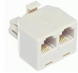
Two devices with modular plugs can be connected to one modular socket using these modular double adaptors. Standard wiring configuration is straight-through. Special wiring configurations are also available.
