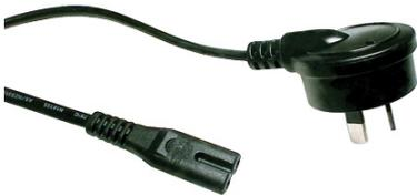
2-core light duty power cord as used on some small appliances. Fitted with IEC-C7 (figure-8) connector and Australian 2-pin right-angle mains plug with insulated pins compliant with AS/NZS3112. Electrical Safety Authority Approved.
