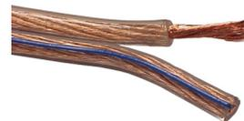
Quality high grade, heavy duty figure-8 speaker cable with transparent PVC jacket. Blue trace-line on one conductor provides easy identification to avoid polarity-reversals during installation. (7x37)259/0.12mm<sup>2</sup> (12AWG) twisted conductors. Supplied on 100 metre, strong polypropylene reels with count-down metre-marking.
