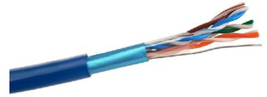
FTP (Foil Twisted Pair) Cat5e cable for premises wiring and applications where shielded cable is required. 4 twisted pairs with solid copper conductors suitable for IDC terminations to patch panels and wall jacks. Conductors are wrapped with aluminium foil shield and Mylar tape. Tinned drain wire. Available in durable 305 metre 5-ply pull-boxes Count-down metre-marking.
