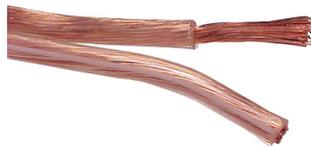
Quality extra heavy duty figure-8 speaker cable with transparent PVC jacket. White trace-line on one conductor provides easy identification to avoid polarity-reversals during installation. 2 x 79/0.20mm<sup>2</sup> (13AWG) conductors. Supplied on 100 metre, strong polypropylene reels with count-down metre-marking.
