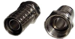
F-type crimp plug for RG6/U quad-shield coaxial cable. Suitable for Digital-TV, CCTV/Security Camera, CATV, SATV and other low-loss applications. Attach using our coaxial cable stripper and professional ratchet crimp tool T0038 using the 0.324" hexagonal die.
