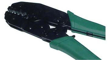
These precision hand crimp tools employ a ratchet action ensuring correct crimping pressure is applied for reliable, trouble-free crimping of coaxial cable plugs. Tool T0038 suits our BNC RG59/U crimp plugs. Tool T0039 is compatible with both our BNC RG59/U crimp plugs and our F-type RG6/U connectors.
