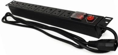
1RU rack mounted power distribution board to suit 19" rack cabinets and wall mounts. 8 x standard 10 Amp Australian AS/NZS mains outlets. 1.8 meter flex cord IEC-C14 inlet. On/off switch and overload switch.
