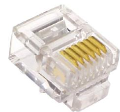
6P modular plug with slots to accommodate pins 1 and 8 of an 8P8C socket. The slots allow greater compatibility with 8P8C sockets. Plugs with 50µ", 30µ", 15µ" or 6µ" gold plated contacts are available. Packed in bags of 20, 50, 100 or 1,000. Plugs for stranded or solid conductors with round or flat cord entry are available.
