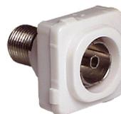
PAL TV connector as used for analogue or digital TV, set-top boxes and VCR connections. F-connector on rear for easy coaxial cable hook-ups. Compatible with our P4600 series Flush Plates and most standard Australian flush plates. PAL connectors are also known as Belling Lee connectors or IEC60169-2 connectors. Available in individual Datamaster® zip-top bags or boxes of 40 pieces.
