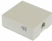
Side entry surface mount voice grade modular socket. Snap-on cover provides access to screw terminals for connection of wires. Double sided tape included for easy installation. Dimensions 50(W) x 57(H) x 20(D)mm.
