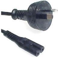
2-core light duty power cord as used on some small appliances. Fitted with IEC-C7 (figure-8) connector and Australian 2-pin mains plug with insulated pins compliant with AS/NZS3112. Electrical Safety Authority Approved.
