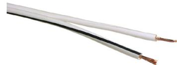
Suitable for speakers and other low voltage applications. Black trace-line on one side of the PVC jacket provides an easy means of identifying the (+) and (-) conductors, eliminating polarity-reversals during installation. Each conductor has 14 strands of 0.20mm<sup>2</sup> diameter copper wire giving an overall conductor-size of 21AWG. PVC jacket OD is 2 x 2.0mm<sup>2</sup>. Standard jacket colours are white and grey. Supplied on 100, 250 and 500 metre strong polypropylene reels.
