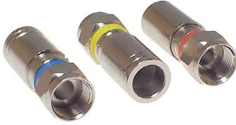
Datamaster's high performance F-type compression connector for trouble free professional water-proof coaxial connections. Available to suit RG59/U or RG6/U dual-shield and RG6/U quad-shield cables. Colour coded bands are used to identify connector/cable compatibility. For best performance use only copper-clad steel cable. Attach using our coaxial cable stripper and professional ratchet compression connector crimp tool T0040.
