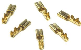
H1130 insulation displacement quick connect crimps, used for connection of insulated line cord conductors to telephone plug types 603, 604, 605, 606 and 615. Single form, packed in poly bags of 10. Also available in continuous form 20K reels.
