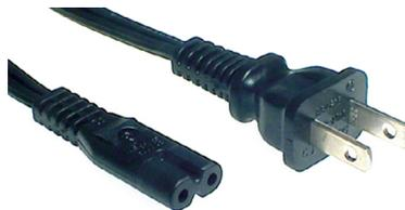
For 110V use. 2-core light duty 18AWG figure-8 power cord as used in U.S.A. for some small appliances. Fitted with IEC-C7 (figure-8) connector and 110V U.S.A. 2-pin mains plug.
