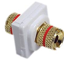
Speaker connectors for Australian flush plates. Front and rear terminals suit either banana plug or screw down termination of speaker wires. Gold finish for corrosion resistance. Ideal for surround sound speaker hook-ups. Compatible with our P4600 series Flush Plates and most standard Australian flush plates. Available in individual Datamaster® zip-top bags or boxes of 30 pieces.
