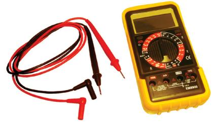
Auto ranging digital multimeter suitable for measuring voltage, current, resistance, capacitance, frequency, temperature and diode/continuity tests. Features a 3½ digit LCD, a data-hold button, a rotary switch for function selection, over-range indication, polarity indication and an inbuilt fuse to protect the meter from damage.
