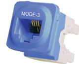
Datamaster's RJ45 8P4C IDC jack with 2 IDC connections per contact allowing easy line-in and line-out for typical alarm dialler applications. Compatible with our P4600 series flush plates and most standard Australian flush plates. Also suits our P4611 Surface Boxes. Rear termination with 110 or Krone IDC impact tool. Available in individual Datamaster® zip-top bags or in reusable buckets of 50 pieces which include a bonus impact safety chassis for safe and speedy termination.
