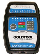
Troubleshoot R45 UTP & STP Lan Cables. The Auto mode makes a single pass over the cable and gives a pass/fail result. The fail result will indicate the type of failure and affected pins/wires. Step mode steps through each wire independently.
