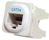
Datamaster's premium RJ45 Cat5e IDC data jack. Compatible with our P4600 series flush plates and most standard Australian flush plates. Also suits our P4611 Surface Boxes. Rear termination with 110 or Krone IDC impact tool. Combined T568A & T568B colour coding for easy installation. Includes a bonus impact safety chassis for safe and speedy termination.
