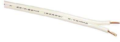
General purpose figure-8 cable suitable for speakers, security systems and other low voltage applications. Printing on one conductor provides easy identification to avoid polarity-reversals during installation. Each conductor has 24 strands of 0.20mm<sup>2</sup> diameter copper wire giving an overall conductor-size of 0.75mm<sup>2</sup> (20AWG). Standard jacket colour is white. Supplied on 100, 250 and 500 metre strong polypropylene reels.
