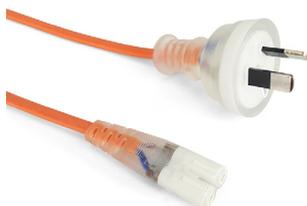
2-core light duty power cord as used on some small appliances. Fitted with IEC-C7 (figure-8) connector and Australian 2-pin mains plug with insulated pins compliant with AS/NZS3112. Orange coloured flex and transparent mains plug & IEC connector as required for medical equipment applications. Electrical Safety Authority Approved.
