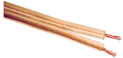
High quality Oxygen Free Copper (OFC) speaker cable for excellent performance. The flat edge on one side of the transparent PVC jacket and printing on one conductor provide easy identification to avoid polarity-reversals during installation. Each conductor has 189 strands of 0.10mm<sup>2</sup> diameter Oxygen Free Copper (twisted in 7 groups of 27) giving an overall conductor-size of 1.5mm<sup>2</sup> (approx 15AWG). Supplied on 100 metre roll with count-down metre marking.
