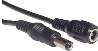
Output cord converter with injection molded DC plug and socket. Convert the existing output plug of a power supply to a different type, size or polarity. Cross-over version reverses polarity from centre-positive to centre-negative or centre-negative to centre-positive whilst either maintaining existing plug type and size or converting to another. Standard length is 130mm overall and standard construction is 20AWG.
