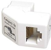
Right-angle Cat5e or Cat6 coupler for use with keystone patch panels or keystone wall plates. Allows ready-made patch cords to be used in fixed installations eliminating the use of solid cable, IDC terminations and tools. Can also be fitted to Australian HPM and Clipsal flush plates by using Clipsal and HPM keystone bezels (DATAMASTER P4590 Clipsal and P4592 HPM) The 1-1 wiring configuration is compatible with both T568A and T568B wiring schemes. Colour is white.
