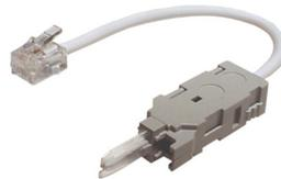
Test cord fitted with IDC type plug and 6P2C modular plug. For connection of test butts or other equipment to Krone MDF or IDF. 100mm long cord.
