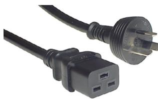
As used on rack mounted power boards. Fitted with a female IEC-C19 connector and an Australian 10 Amp or 15 Amp 3-pin mains plug with insulated pins compliant with AS/NZS3112. Electrical Safety Authority Approved.
