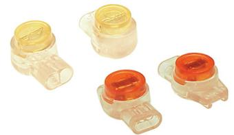
Gel filled, IDC, insulated, butt connector for 2 or 3 solid copper conductors of 19 to 26 AWG having maximum insulation OD of 2.08mm. Simple crimp-connection using our gel-connector crimp tool T0037 for fast, easy and reliable installation. Contains moisture resistant sealant, rated to IP67 (dust resistant and immersible up to 1 metre).
