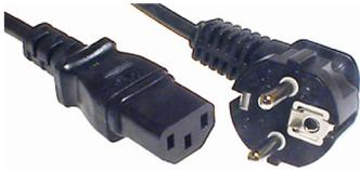
10 Amp AC power cord as used on most European computers and office equipment. Fitted with an IEC-C13 connector and a right-angled 230V earthed European Schuko mains plug.
