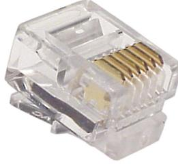
Generally used for termination of line cords. Plugs with 50µ", 30µ", 15µ" or 6µ" gold plated contacts are available. Packed in bags of 5, 20, 50, 100 or bulk. Plugs for stranded or solid conductors with round or flat cord entry are stocked.
