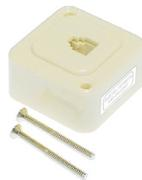
Compact surface mount voice grade modular socket. Recessed screws allow fast and easy fixing to almost any surface. Wires are connected by screw terminals. Beige colour suits most environments. Dimensions 44(W) x 44(H) x 25(D)mm.
