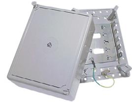
Grey coloured wall-mounted plastic distribution box containing mounting brackets for 10-pair IDC-type connection modules (available separately). Cable entry holes in rear and cable entry cut-outs on all 4 sides. Four moveable jumper rings and record-card included.
