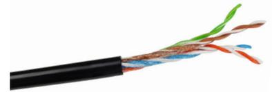
Cat-5e cable for outdoor and underground burial. Gel-filled jacket to prevent water ingress. 4 twisted pairs with solid copper conductors suitable for IDC terminations. Supplied on 300 metre reels. Count-down metre-marking.
