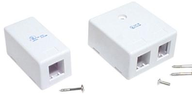
Side entry surface mount boxes to accept our standard keystone 110 jacks or other keystone connectors. Snap-on cover for easy installation and access to wiring. Single and duplex versions available. Double sided tape included for easy installation. The standard colour is white. Supplied unloaded without keystone jacks.
