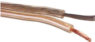
Quality figure-8 speaker cable with transparent PVC jacket. One conductor is tinned copper and the other is bare copper with a white trace-line providing easy identification and to avoid polarity-reversals during installation. 2 x 41/0.20mm<sup>2</sup> (16AWG). Supplied on 100 metre, strong polypropylene reels with count-down metre-marking.
