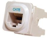
Datamaster's premium RJ45 Cat6 IDC data jack. Compatible with our P4600 series flush plates and most standard Australian flush plates. Also suits our P4611 Surface Boxes. Rear termination with 110 or Krone IDC impact tool. Combined T568A & T568B colour coding for easy installation. Available in individual Datamaster® zip-top bags or buckets of 50 pieces which include a bonus impact safety chassis for safe and speedy termination.
