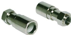
Datamaster's high performance F-type compression connector for trouble free professional water-proof coaxial connections to RG11/U quad-shield coaxial cable. For best performance use only copper-clad steel cable. Attach using our professional ratchet compression connector crimp tool T0041.
