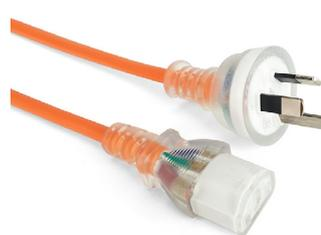
A 3-core general duty power cord fitted with IEC-C13 connector and Australian 3-pin mains plug with insulated pins compliant with AS/NZS3112. Orange coloured flex and transparent mains plug & IEC connector as required for medical equipment applications. Also see our K3755ORA medical equipment cord with a left-hand right-angle socket. Electrical Safety Authority Approved.
