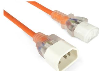
A 3-core IEC extension power cord fitted with female IEC-C13 and male IEC-C14 connectors. Orange coloured flex and transparent IEC connectors as required for medical equipment applications. Electrical Safety Authority Approved.
