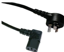
3-core flex fitted with a right-angle 3-pin Australian mains plug with insulated pins compliant with AS/NZS3112 and a left-hand right-angle IEC-C13 connector. Electrical Safety Authority Approved.
