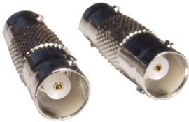
BNC coupler enables two coaxial cables fitted with male BNC plugs to be coupled together. Knurled centre section provides grip whilst connecting or disconnecting BNC plugs. Can also be used as a gender changer.
