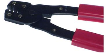
This quality metal crimp tool is designed for accurate termination of H1130 insulation displacement quick connect crimps that are used for connection of insulated line cord conductors to telephone plug types 603, 604, 605, 606 and 615. Also suitable for crimping our insulation displacement Y-terminals and other 14-28AWG insulated and non-insulated connectors and pins. A handle operated cord cutter is incorporated.
