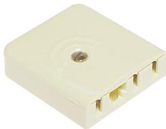
Suitable for security devices, diallers, modems and other auxiliary equipment. Accepts 604, 605 or 606 telephone plugs. Often referred to as a mode-3 socket. Cams allow each terminal pair to be switched or unswitched when plug is withdrawn.
