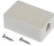
Half sized surface mount voice grade modular socket designed to be fixed to skirting boards or architraves. Snap-on cover provides access to screw terminals for connection of wires. Double sided tape included for easy installation. Dimensions 31(W) x 50(H) x 20(D)mm.
