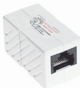
Cat5e coupler can be used to link 2 patch cords together or as a gender changer. The 1-1 wiring configuration is compatible with both T568A and T568B wiring schemes. Colour is white.
