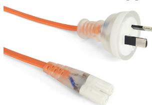
2-core light duty power cord as used on some small appliances. Fitted with IEC-C7 (figure-8) connector and Australian 2-pin mains plug with insulated pins compliant with AS/NZS3112. Orange coloured flex and transparent mains plug & IEC connector as required for medical equipment applications. Electrical Safety Authority Approved.
