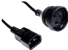
10 Amp 3-core power cord fitted with standard Australian mains socket and an IEC-C14 connector. Suitable for connection of a device fitted with a standard mains plug to an IEC-C13 connector. Typically used to connect a PC to a UPS. Electrical Safety Authority Approved.
