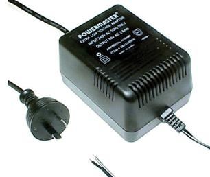
In-line AC adaptor with 48 Watt maximum capacity. Ventilated case. The 16V model feature a flush mounted LED indicator. The AC input cord is fitted with mains plug and insulated pins compliant with AS/NZS3112. Dimensions 110(L) x 83(W) x 65(H) mm. Electrical Safety Authority Approved.
