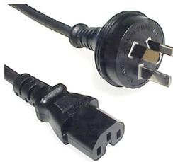
A 10 Amp AC high temperature (120°C) appliance cord with elastomer flex as required by computer servers and hot kitchen appliances. Fitted with high-temperature, notched-type IEC-C15 appliance connector and an Australian 3-pin mains plug with insulated pins compliant with AS/NZS3112. Electrical Safety Authority Approved.
