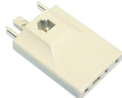
The 616M combines a 605 plug and a 610 socket, with either 6P4C (RJ11) or 8P4C (RJ45) modular socket. Updated design has front entry modular socket for easier use with side mounted wall sockets. Parallel wiring and mode-3 wiring versions are available. Blister pack model includes reducer to suit either RJ11 or RJ45. Custom wiring configurations and colours can also be made if required.
