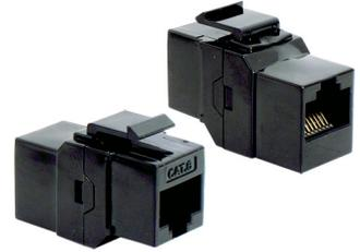
Cat6 coupler for use with Keystone patch panels, and flush plates. Allows ready-made Cat6 patch cords to be used in fixed installations eliminating the use of IDC terminations and tools. Can also be fitted to Australian HPM and Clipsal flush plates by using Clipsal and HPM keystone bezels (DATAMASTER P4590 Clipsal and P4592 HPM) The 1-1 wiring configuration is compatible with both T568A and T568B wiring schemes. Colour is black.
