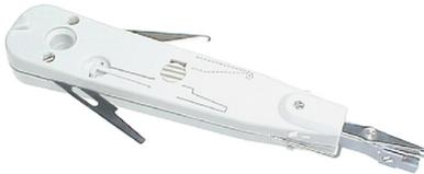
For IDC connections, P8710 disconnect modules or any Krone type terminals. Simultaneous cut & terminate operations. Fold-out hook and screwdriver accessories. The sensor prevents angled termination and also helps with double jumpering by cutting the second wire before the first wire. On/Off cutting function. Terminate wires with a diameter of 0.4 - 0.9mm (20-27AWG) and insulation of 0.70 to 1.90mm. Not suitable for 110 type IDC terminals.
