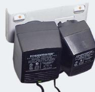
This example shows an attempt to use two wide power supplies in the same double power point. Both the power supplies are displaced. Neither can be inserted correctly and neither power supply will operate safely.
