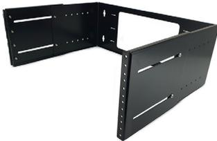
Wall mount bracket for the installation of patch panels or other 19" rack mounted equipment. 1RU, 2RU, 4RU and 8RU models available. Hinged for easy access to wiring. Panel bolts included. Depth is adjustable between 227mm and 352mm. Black colour.
