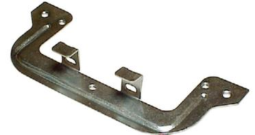
Datamaster's Galvanised metal bracket for fitting standard Australian flush plates into plaster board. Wall lugs are factory set to suit 12mm thick plaster board but can be adjusted to suit 6mm thick fibro. Dimensions and hole centres suit our P4600 series flush plates and most other standard Australian switch plates.
