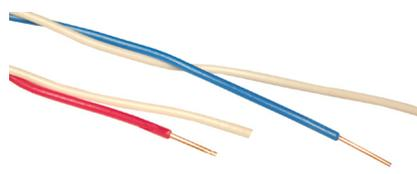
PVC insulated annealed copper jumper wire primarily designed for jumpering or hook-ups on communications distribution frame IDC modules. Outer diameter 1.08mm. Conductor diameter 0.5mm. Conductor resistance <98.0Ω/km. Available on 250 metre wooden reels with either Red/White or Blue/White pairing.
