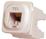
Datamaster's 6P4C IDC jack for telephone applications. 2 IDC connections per contact allowing easy loop-in, loop-out for typical voice applications. Compatible with our P4600 series flush plates and most standard Australian flush plates. Also suits our P4611 Surface Boxes. Rear termination with 110 or Krone IDC impact tool. Available in individual Datamaster® zip-top bags or in reusable buckets of 50 pieces which include a bonus impact safety chassis for safe and speedy termination.
