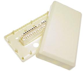
Ivory coloured surface-mount distribution box with cable entry holes in rear and cable entry cut-outs on all 4 sides. Contains a 10-pair IDC module constructed of high-impact fire-resistant PBT material with corrosion resistant 5.0 micron silver-plated terminals. Terminate wires using our T0059 impact tool (or any impact tool designed for termination of Krone-type IDC terminals). Supports pair-disconnect function if appropriate test plug is inserted. Dimensions 164(H) x 85(W) x 36(D)mm.
