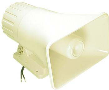
15 watt horn speaker suitable for connection to the K3507 Tone Ringer or to the K3509 Universal Loud Sounding Alarm. The 350mm figure-8 cable has tinned ends for easy connection. IP4, splash-proof. Colour is white.
