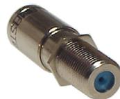
Datamaster's high performance female F-Type compression connector for trouble free professional water-proof coaxial connections. Blue coloured tip indicates compatibility with RG6/U quad-shield coaxial cable. Attach using our coaxial cable stripper and professional ratchet compression connector crimp tool T0040.
