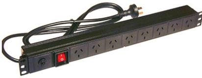
1RU rack mounted power distribution board to suit 19" rack cabinets and wall mounts. 8 x standard 10 Amp Australian AS/NZS mains outlets. 1.8 meter flex cord and 10 Amp Australian mains plug. On/off switch and overload switch.
