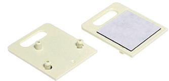
Self adhesive backing plate to eliminate the requirement to use screws when mounting 610 or 611 sockets to any flat, clean surface. Our 610 or 611 sockets simply snap-on to the backing plate.
