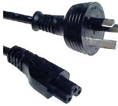
3-core general duty power cord as used on some compact Switch Mode Power Supplies (laptop computers) and small appliances. Fitted with IEC-C5 connector and Australian 3-pin mains plug with insulated pins compliant with AS/NZS3112. Electrical Safety Authority Approved.
