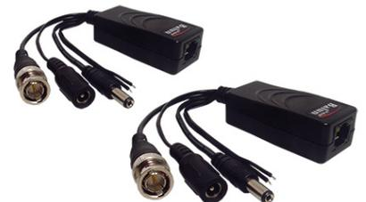
Used to carry CCTV video signal, power feed and data for PTZ over Cat5e or Cat6 cable. Passive design transmits colour video up to 400 metres, 12V or 24V, power feed up to 250 metres and PTZ data up to 300 metres. Integrated surge protection. Male BNC for video connections, male/female barrel plug/socket for power feed, RJ45 modular socket for connection to the Cat5e or Cat6 cable and tinned ends for PTZ data connection. Packed in a blister pack set of two.
