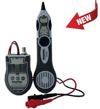
Wiring system tester, connection map test for discontinuity, short circuit, reversed pairs, crossed pairs, wire tracing, cable continuity, polarity and verifying a line. Possibility of identifying & tracing wires or cables with no damage to insulation. Max. 1km cable length, min. receiver distance: 60cm. Signal frequency 500-781Hz, signal frequency 500Hz-781Hz
