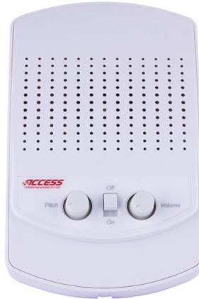
Robust extension tone ringer with volume and pitch controls and an on/off switch. Connection to the exchange line is via either screw terminals or modular socket. Unit has a built-in speaker. An optional 15 watt horn speaker (connected via screw terminals) is available for more directional signalling of incoming calls. Maximum volume 98dB. This unit has a REN of 1.9. Dimensions 115(W) x 155(H) x 35(D)mm.
