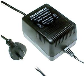
In-line AC adaptor with 48 Watt maximum capacity. Ventilated case. The 16V model feature a flush mounted LED indicator. The AC input cord is fitted with mains plug and insulated pins compliant with AS/NZS3112. Dimensions 110(L) x 83(W) x 65(H) mm. Electrical Safety Authority Approved.
