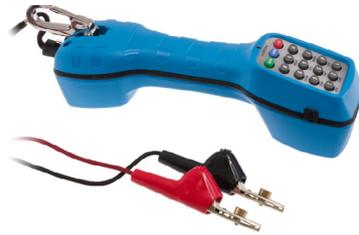
Test Telephone with 2-way hands-free speaker, adjustable volume switch, line polarity check and monitor/talk switch. Tone or pulse dialing with last number redial and 12 memories. ABS housing with belt clip and durable coiled cord. Measures 260(L) x 70(W) x 89(H)mm. Weight 560g.
