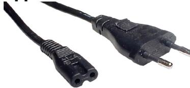
2-core light duty power cord as used on some small appliances for use in Europe. Fitted with IEC-C7 (figure-8) connector and a 2-pin European mains plug.
