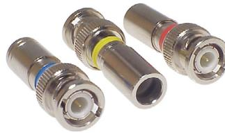
Datamaster's high performance BNC compression connector for trouble free professional water-proof coaxial connections. Available to suit RG59/U or RG6/U dual-shield and RG6/U quad-shield cables. Colour coded bands are used to identify connector/cable compatibility. The 1-piece design suits either solid copper or copper clad steel cable. Attach using our coaxial cable stripper and professional ratchet compression connector crimp tool T0040.
