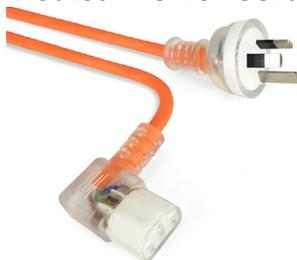
A 3-core general duty power cord fitted with a left-hand right-angle IEC-C13 connector and Australian 3-pin mains plug with insulated pins compliant with AS/NZS3112. Orange coloured flex and transparent mains plug & IEC connector as required for medical equipment applications. Electrical Safety Authority Approved.
