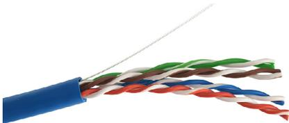
Our quality Cat-5e stranded conductor cable is suitable for assembly of patch cords. 4 twisted pairs 24AWG with 7/0.20mm<sup>2</sup> stranded conductors. Available on 100 and 305 metre reels or in durable 305 metre 5-ply pull-boxes. Count-down metre-marking.
