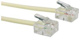
2 conductor line cord with 6P2C RJ11 modular plugs on each end. Standard wiring is cross-over to suit most voice applications.
