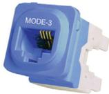
Datamaster's RJ45 8P4C IDC jack with 2 IDC connections per contact allowing easy line-in and line-out for typical alarm dialler applications. Compatible with our P4600 series flush plates and most standard Australian flush plates. Also suits our P4611 Surface Boxes. Rear termination with 110 or Krone IDC impact tool. Available in individual Datamaster® zip-top bags or in reusable buckets of 50 pieces which include a bonus impact safety chassis for safe and speedy termination.
