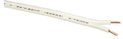
General purpose figure-8 cable suitable for speakers, security systems and other low voltage applications. Printing on one conductor provides easy identification to avoid polarity-reversals during installation. Each conductor has 24 strands of 0.20mm<sup>2</sup> diameter copper wire giving an overall conductor-size of 0.75mm<sup>2</sup> (20AWG).
