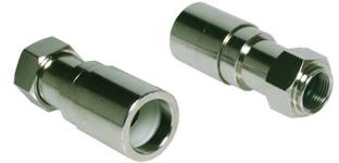
Datamaster's high performance F-type compression connector for trouble free professional water-proof coaxial connections to RG11/U quad-shield coaxial cable. For best performance use only copper-clad steel cable. Attach using our professional ratchet compression connector crimp tool T0041.
