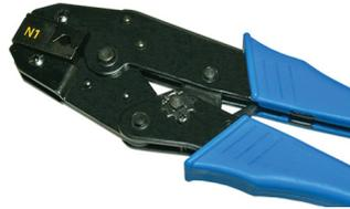
This precision crimp tool is designed specifically for Cat6 shielded modular plugs only.
