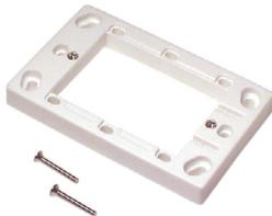
Datamaster's 13mm deep block for surface mounting standard Australian flush plates. Suits our P4600 series flush plates and most other standard Australian switch plates. Supplied with screws for fitting flush plate. Dimensions 118(W) x 75(H) x 13(D)mm.
