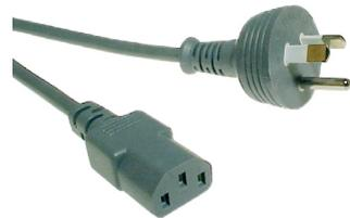
Power cord fitted with IEC-C13 connector (straight or right-angled) and Australian Special Purpose 3-pin mains plug with round earth pin and insulated active and neutral pins compliant with AS/NZS3112. Applications include lighting, exhaust fans, cash registers or IT equipment which may be connected to a special purpose power circuit. Electrical Safety Authority Approved.
