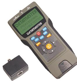
Professional LAN cable tester with advanced backlit LCD. Tests and displays exact pin-to-pin wiring configuration of LAN cables, modular telephone cables and coaxial cables. Tests and displays length of LAN or coaxial cables. With remote terminator (ID #01) for near-end/far-end testing of installed network cables on site, 2 x F-type to BNC coax adaptors, 2 x 8P to 6P modular reducers and 9V battery.
