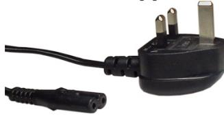
2-core light duty power cord as used on some small appliances for use in UK, Hong Kong or Singapore. Fitted with an IEC-C7 (figure-8) connector and a UK 3-pin mains plug with integrated 3 Amp fuse. BS Approved.
