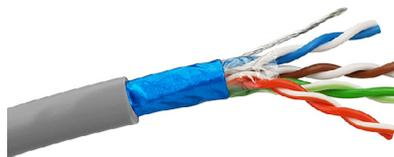
Shielded FTP (Foil Twisted Pair) Cat5e cable with 7/0.20mm<sup>2</sup> stranded conductors in 4 twisted pairs. Conductors are wrapped with aluminium foil shield and mylar tape. Tinned 7/0.30mm<sup>2</sup> drain wire. Count-down metre-marking.
