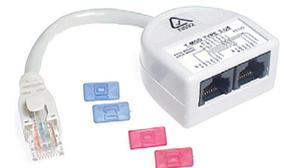
Cat5e splitters enable two different devices to share the same cable. They are usually used in pairs, one at the outlet and one at the patch panel. The 100mm cord allows use in high-density panels. Several wiring configurations are available to split the four pairs to suit different applications. Packed in a zip-lock bag. Colour is Ash.
