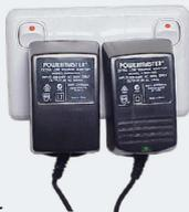
In an attempt to use one wide plus one narrow power supply in the same double power point, only one will be able to be fully inserted and the other power supply will not work. This example shows the wide power supply displacing the "narrow" power supply and preventing it from operating safely.
