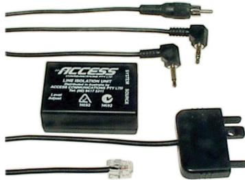
Compact LIU allows any audio device having an earphone or line-out socket to be connected to any compatible Key Telephone or PABX system to provide music to calls that are placed on hold. Incorporates a recessed potentiometer to adjust volume level. The Source cords are 600mm long. The length of the System cord is shown in the table below.
