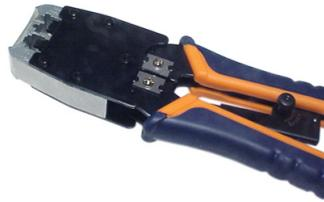
Two individual dies allow accurate termination of 6 and 8 position modular plugs. Jaw design distributes equal pressure to all contacts simultaneously. Ratchet operation ensures excellent insulation penetration and cord strain relief.
