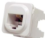
Datamaster's voice grade RJ45 8P4C IDC jack with 2 IDC connections per contact allowing easy loop-in, loop-out for typical voice applications. Compatible with our P4600 series flush plates and most standard Australian flush plates. Also suits our P4611 Surface Boxes. Rear termination with 110 or Krone IDC impact tool. Available in individual Datamaster® zip-top bags or buckets of 50 pieces which include a bonus impact safety chassis for safe and speedy termination.
