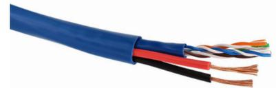
Composite cable containing a Cat-5E cable plus two 24/0.20mm<sup>2</sup> conductors (one red, one black) for power feed. Suitable for IP CCTV/Security-camera use where a separate power feed is required for the camera and/or pan/tilt/zoom mechanism. Outer jacket is flexible blue PVC with count-down metre-marking. Available on 100 metre or 200 metre wooden reels.
