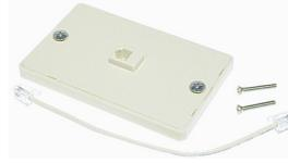
Wall phone bracket for easy installation of telephones that have standard modular wall mountings. The line is connected from bracket to phone by a 160mm long modular cord. Bracket has two studs onto which the phone slides. Fits standard Australian electrical switch plate installation hardware. Off-white colour to match Telstra T200/400 telephones. Dimensions 76(W) x 119(H) x 9(D)mm.
