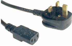
10 Amp AC power cord as used on most U.K. Hong Kong or Singapore computers and office equipment. Fitted with an IEC-C13 connector and a 230V 3-pin U.K. mains plug with integrated 13 Amp fuse.
