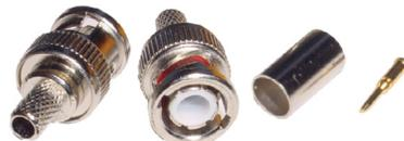
BNC crimp plug suitable for RG59/U or RG6/U coaxial cables. The 3-piece design has a separate crimp-pin for trouble free connection to either solid copper or copper-clad steel cables. Attach using our coaxial cable stripper and professional ratchet crimp tool T0038 or T0039 using the 0.068" hexagonal die for the pin and the 0.255" or 0.262" hexagonal die for the sleeve.
