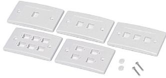
Flush type plates to accept our standard keystone jacks, couplers and F-connectors. Fits standard Australian electrical switch plate installation hardware and screw centres, making it perfect for easy flush installation on gyprock or fibro cavity walls. Supplied unloaded without keystone jacks. Dimensions 70(W) x 114(H) x 6(D)mm.
