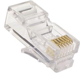
Similar to the standard 6 position modular plug but has a long body as required to mate with deeply recessed modular sockets. Plugs with 50µ", 30µ" or 15µ" gold plated contacts are available. Packed in bags of 20, 50, 100 or 1000. Plugs for stranded or solid conductors with round or flat cord entry are available.
