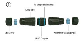
Accessories: 2pcs End Covers, 2pcs long tubes, 1 pc RJ45 Coupler, 2pcs O-shape sealling rings, 2pcs waterproof sealing plugs.
