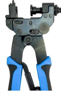
These precision hand crimp tools employ a ratchet action ensuring correct crimping pressure is applied for reliable, trouble-free compression of our P0720 series waterproof BNC, RCA, PAL and F-type coaxial connectors. Adjustable compression depth. Tool T0040 is compatible with RG6/U and RG59/U coaxial cables and has adaptors to suit F-type and Female connectors. Tool T0041 is suitable for only F-type connectors on RG11/U coaxial cable.
