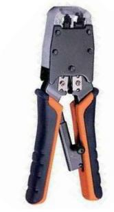
Two individual dies allow accurate termination of 6 and 8 position modular plugs. Jaw design distributes equal pressure to all contacts simultaneously. Ratchet operation ensures excellent insulation penetration and cord strain relief.
