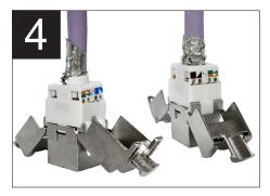
Push the termination cap onto the back of the jack, ensuring the moulded t-piece in the centre of the termination cap marries with the female reciprical in the IDC environment.
