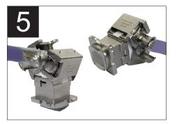
Press both doors of jack to make secure contact with the cable. This will also lock the termination cap onto the IDC is, pushing the conductor wires into the blades. Wrap the conductive foil and drain wire around the cable allowing the clamps to mate with the foil and wire.
