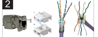
Feed the coductors into the hole from the bottom with the termination cap facing grooves up. Fit the copper wires into colour coded slots, ensuring they slot into the two grooves, so it feeds out past the edge.
