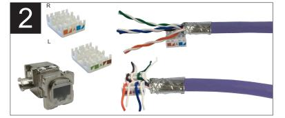
Feed the coductors into the hole from the bottom with the termination cap facing grooves up. Fit the copper wires into colour coded slots, ensuring they slot into the two grooves, so it feeds out past the edge.
