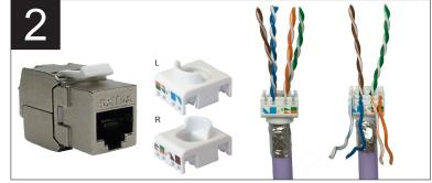
Feed the coductors into the hole from the bottom with the termination cap facing grooves up. Fit the copper wires into colour coded slots, ensuring they slot into the two grooves, so it feeds out past the edge.
