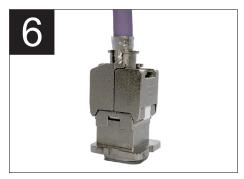
Close the doors of the jack together to complete the mating of the cable to the jack. You will hear a click when it is shut and locks into place. The door clamps should now be touching the foil and drain wire.
