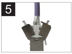
Press both doors of jack to make secure contact with the cable. This will also lock the termination cap onto the IDC is, pushing the conductor wires into the blades. Wrap the conductive foil and drain wire around the cable allowing the clamps to mate with the foil and wire.
