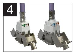
Push the termination cap onto the back of the jack, ensuring the moulded t-piece in the centre of the termination cap marries with the female reciprical in the IDC environment.
